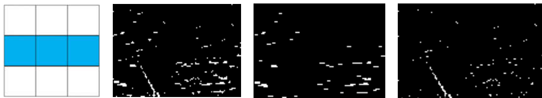
Figure 4. Horizontal wave line points removing: (a) the horizontal filter; (b) the potential towing line points map; (c) the horizontal line points filtered by the horizontal filter; (d) the final result map.
