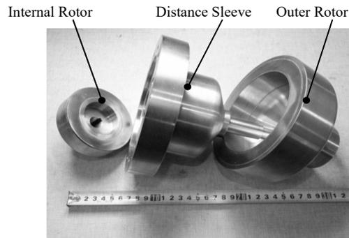
Figure 4. Photo of the magnetic coupling coupler.
