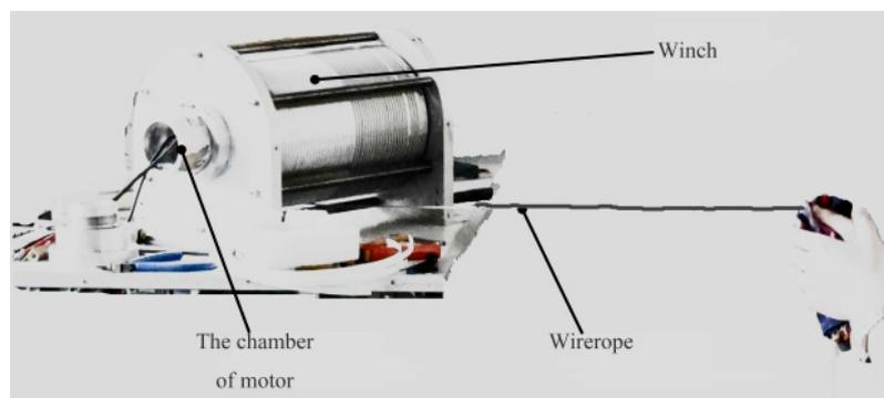
Figure 11. The commissioning of servo winch.
