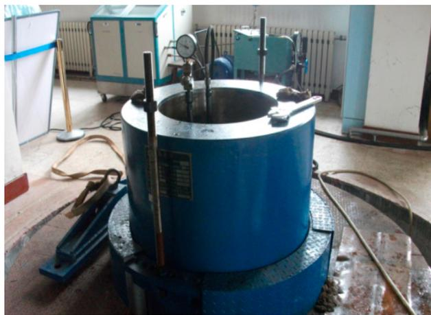
**Figure 12.** The pressure test chamber.
