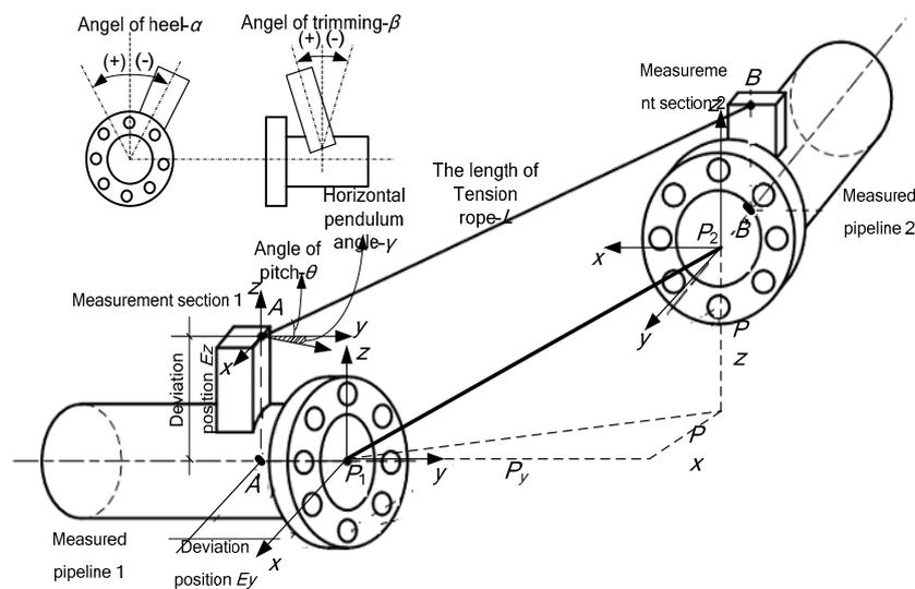
Figure 2. The parameters of relative pipeline poses.
