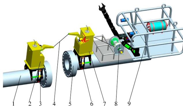
**Figure 1.** The deep-water pipeline pose measurement device. 1, pipeline 1; 2, measurement section I; 3, butting base I; 4, detection rope; 5, pipeline 2; 6, butting base II; 7, measurement section II; 8, winch; 9, ROV (Remote Operated Vehicle).
