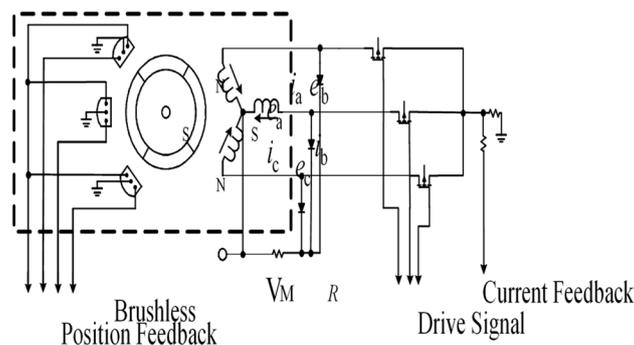
Figure 6. Star type connection of brushless motor.
