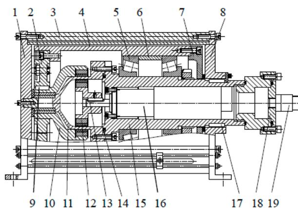
**Figure 3.** Schematic diagram of magnetic coupling winch. 1, left support plate; 2, left drum cover; 3, locating rods; 4, barrel; 5, roller bears; 6, spacer sleeve; 7, right drum cover; 8, right support plate; 9, key joint; 10, outer magnetic rotor; 11, left-hand flange; 12, active magnetic rotor; 13, motor shaft; 14, O-shaped seal; 15, sealed enclosure; 16, motor; 17, fixing key; 18, right cover; 19, watertight cable glands.
