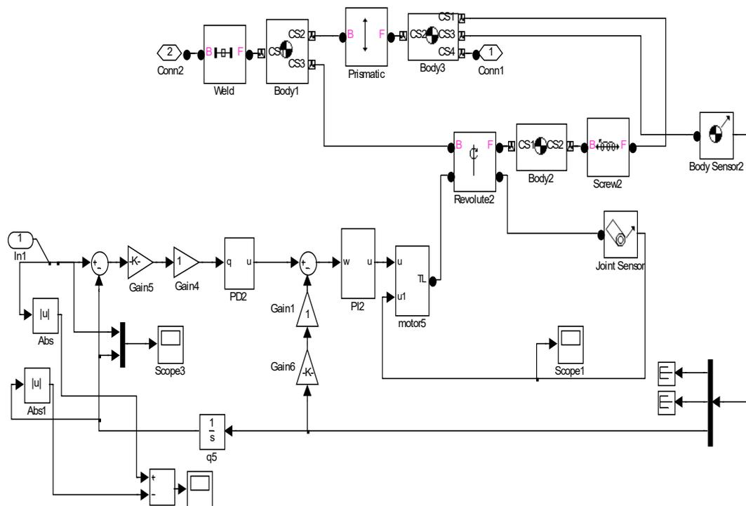
Figure 8. The brushless motor servo control system.
