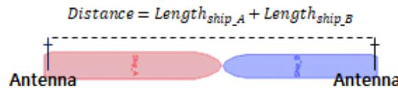
**Figure 4.** Distance the antennae of two vessels when the antennae are installed at the stern, where there is a collision even though the computed distance between the two antenna positions is not zero.
