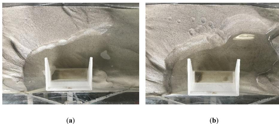
**Figure 4.** Top view of the backfill after the tsunami (run 1): (a)  $t_{pump} = 30$  s; (b)  $t_{pump} = 50$  s. The tsunami passed from left to right. The white object at near side is the abutment. The rightward direction is  $x$  axis, upward direction is  $y$  axis.
