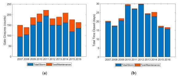
Figure 4. Number of gate closures (a) and total time closed (b) per year for 2007 to 2016.
