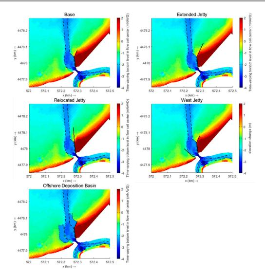
**Figure 9.** Modeled alternatives with initial bathymetry. Dredge template by dashed line, jetty by solid black line, and deposition basins by the dot and dashed line.
