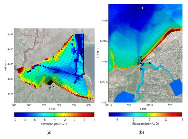
**Figure 6.** (a) Hydrodynamic modeling domain and grid configuration with (solid black line) eastern open boundary (b) detail in vicinity of project site. The wave modeling grid (not shown) covers the same active modeling domain and has a corresponding open boundary. Numbers denote instrument locations. See Table 3 for details.
