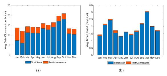
**Figure 5.** Average number of gate closures (**a**) and duration of closures per year (**b**) during each month based on gate closure data from 2007 to 2016.
