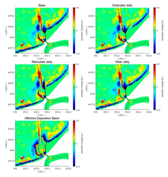
**Figure 10.** Cumulative sedimentation/erosion for modeled period (28 days): WNW Storm. Area of interest/channel limits by dashed line, jetty by solid black line, and deposition basins by the dot and dashed line.
