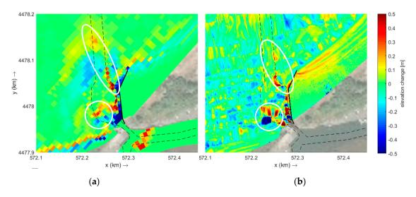
**Figure 8.** (a) Modeled and (b) observed cumulative erosion/sedimentation plot for the Spring 2018 deployment. Channel limits denoted by dashed line.
