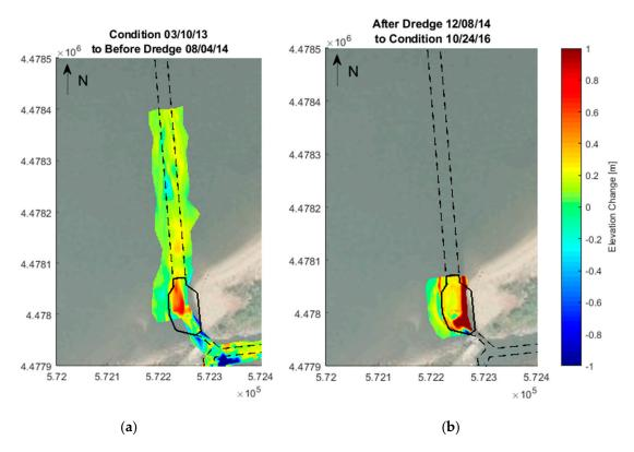
**Figure 3.** Elevation difference plots for two surveys within (**a**) design template footprint represented as a black dotted line and (**b**) partial dredging inlet throat smaller area for volume calculations as black solid line.
