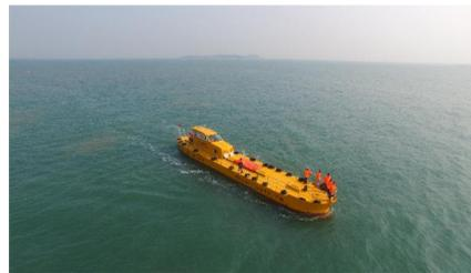
Figure 1. Self-propulsion test of a large-scale ship model at sea.
