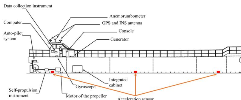
Figure 2. General arrangement of the relevant equipment on the large-scale ship model.
