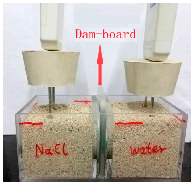
Figure 5. Molecular diffusion and pore tortuosity test device.
