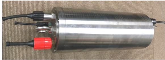
Figure 4. Data control module.
