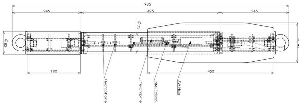
**Figure 5.** Schematic diagram of the single acoustic module.
