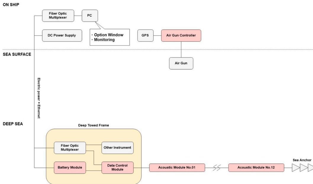
Figure 1. Block diagram of the deep-towed streamer.
