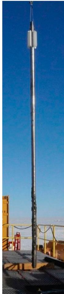
**Figure 20.** WISSARD/Caltech piston corer with sediments packed at lower part [8] (Reproduced with permission from Royal Society, 2016).
