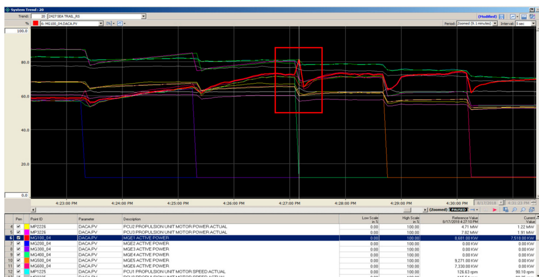
Figure 19. The hunting of the output voltage of generator due to load variation in the actual operation of the ship.
