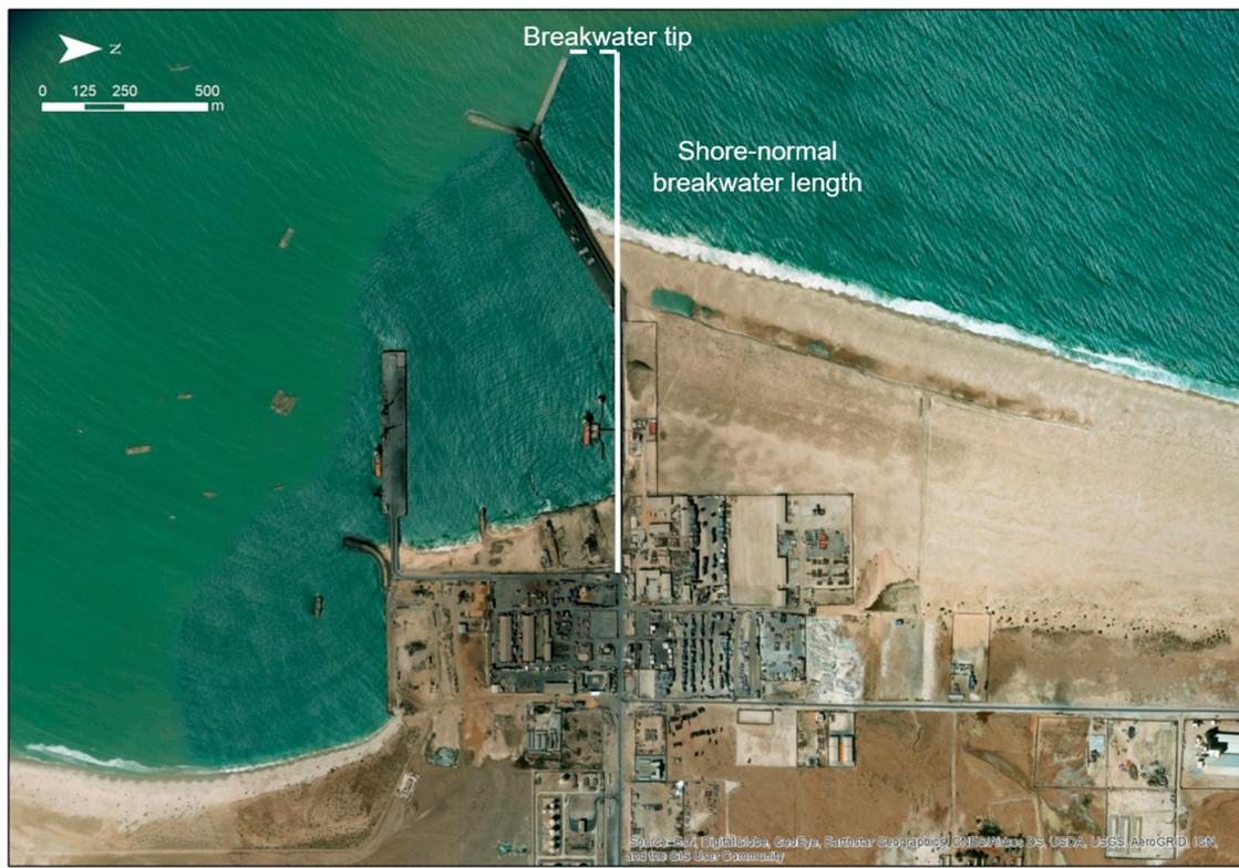
**Figure 8.** Illustration of the method used to determine the shore-normal breakwater length for the Port of Nouakchott (Mauritania).
