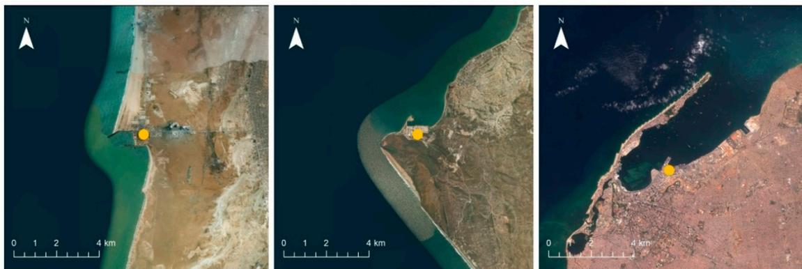
**Figure 7.** Examples of ports with different sheltering settings. Left—open sandy coast (Port of Nouakchott, Mauritania); middle—headland-bay coast (Port of Amboim, Angola); right—coast behind natural barrier (Port of Luanda, Angola).
