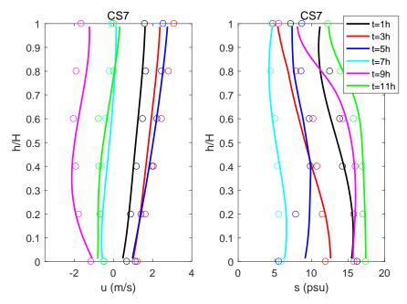
**Figure 5.** Comparison of current speed (*u*) and salinity (*s*) at CS7. (Solid lines: predicted results; Circles: observations).
