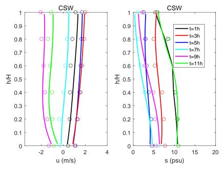
**Figure 4.** Comparison of current speed (*u*) and salinity (*s*) at CSW. (Solid lines: predicted results; Circles: observations).
