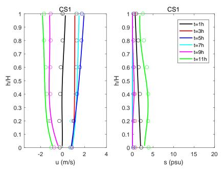
**Figure 3.** Comparison of current speed (*u*) and salinity (*s*) at CS1. (Solid lines: predicted results; Circles: observations).
