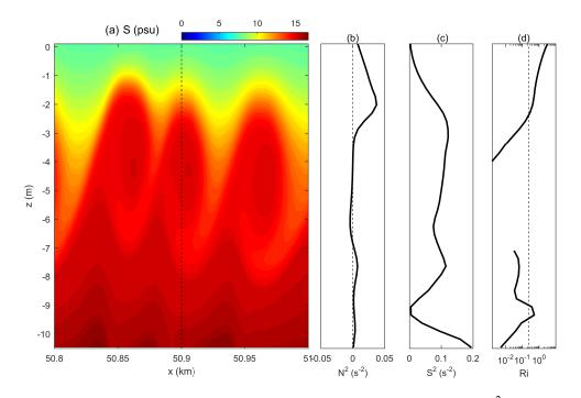
**Figure 7.** Vertical distributions of (**a**) salinity, (**b**) the Brunt-Väisälä frequency ( $N^2$ ), (**c**) the velocity shear ( $S^2$ ) and (**d**) Richardson number (Ri) at t = 7.2 h. (Dashed line in (**a**) represents the location for calculating  $N^2$ ,  $S^2$  and Ri; Dashed line in (**d**) means Ri = 0.25).
