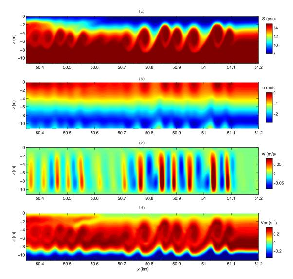
**Figure 12.** Distributions of (a) salinity, (b) streamwise velocity(u), (c) vertical velocity (w) and (d) spanwise vorticity at t = 7.2 h.
