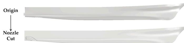
**Figure 8.** Modification of the Athena waterjet model.
