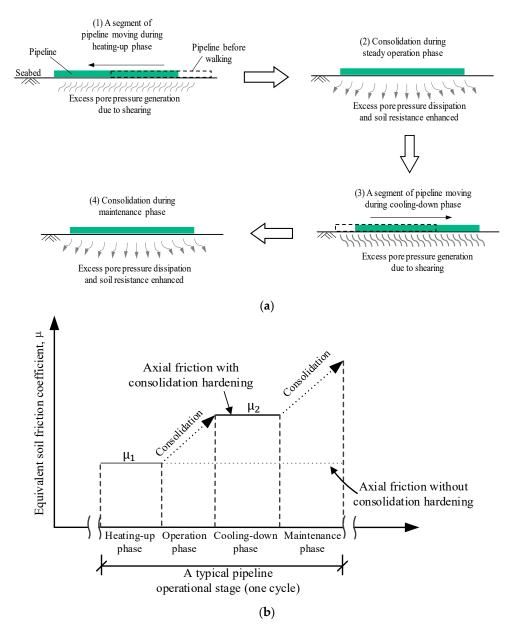
**Figure 1.** Demonstration of responses during pipeline walking: (**a**) Displacement of a segment of pipeline, and (**b**) change in equivalent soil friction due to reconsolidation in a typical operational loading cycle.
