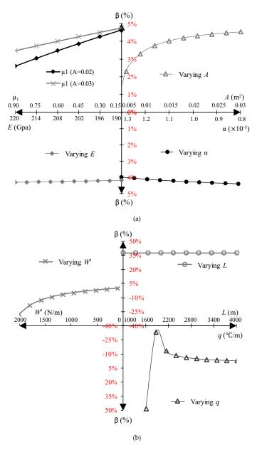
**Figure 8.** Variation of  $\beta$  against different influential factors under thermal transient condition ( $\eta = 1.1$ ): (a) Varying  $\mu$ , *A*, *E*, and  $\alpha$ ; (b) varying *W'*, *L*, and *q*.
