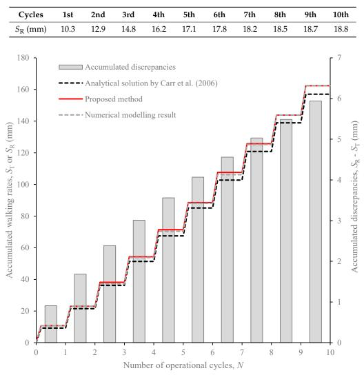
**Table 6.** Pipeline walking rate  $S_{\rm R}$  estimated by the method proposed in this study.
