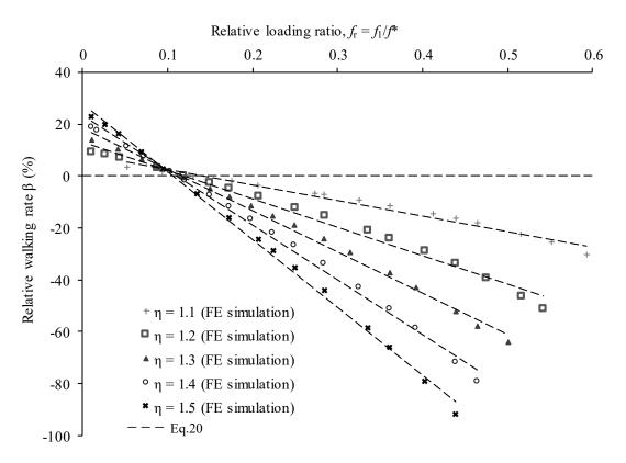
**Figure 12.** Relative walking rate  $\beta$  against relative loading ratio  $f_r$  under thermal transient condition.
