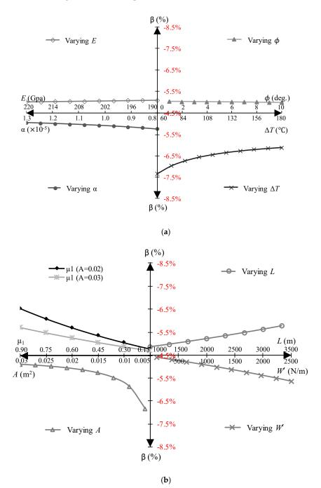
**Figure 7.** Variation of  $\beta$  against different influential factors under downslope condition ( $\eta = 1.1$ ): (a) Varying *E*,  $\phi$ ,  $\alpha$ , and  $\Delta T$ ; (b) varying  $\mu$ , *L*, *A*, and *W*'.
