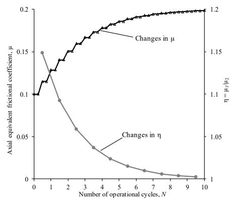
**Figure 14.** Variation of axial equivalent frictional coefficient and corresponding gain in axial friction over 10 operational cycles.
