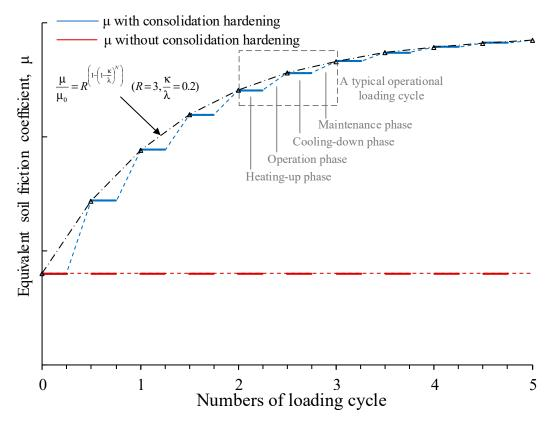
**Figure 4.** Transformation from gain in soil friction against shearing cycles to that against operational loading cycles.
