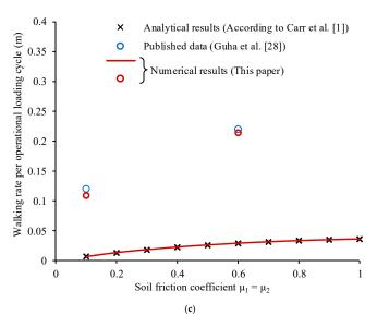
**Figure 5.** Comparison of pipe walking from numerical analysis and conventional analytical solutions (Carr et al., 2006) under: (a) SCR tension condition; (b) downslope condition; (c) thermal transient condition.
