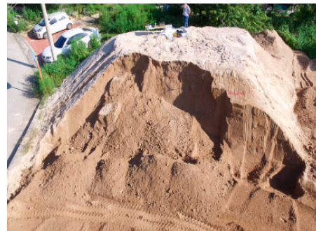
Figure 7. Slope failure after cutting.
