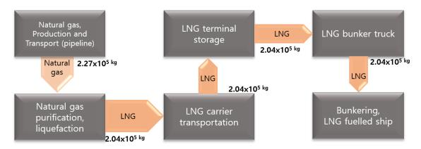
Figure 7. WtT LCA model for LNG fuel.
