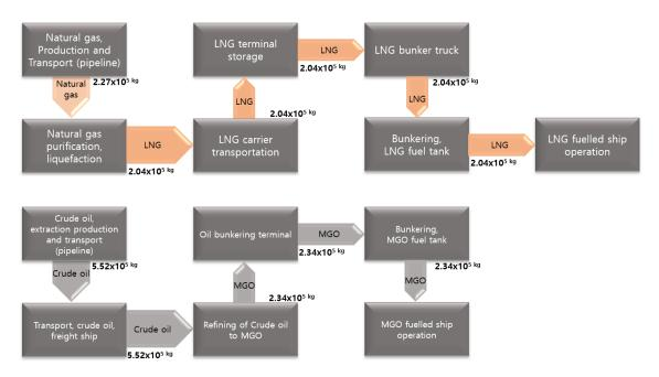
Figure 10. WtW LCA model for LNG fuel and MGO fuel.
