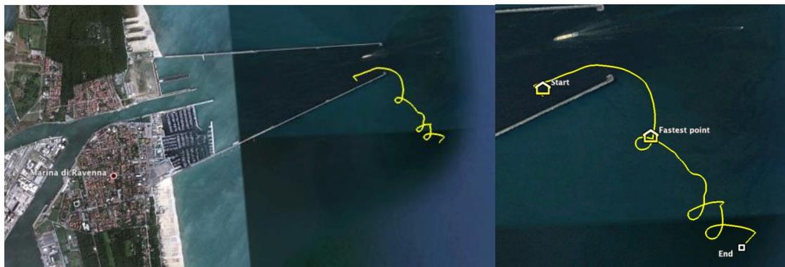
**Figure 9.** Example of route followed during one of the test sessions: strong acceleration and repeated rotations made it possible to investigate the effect of self-generated waves on the hull.
