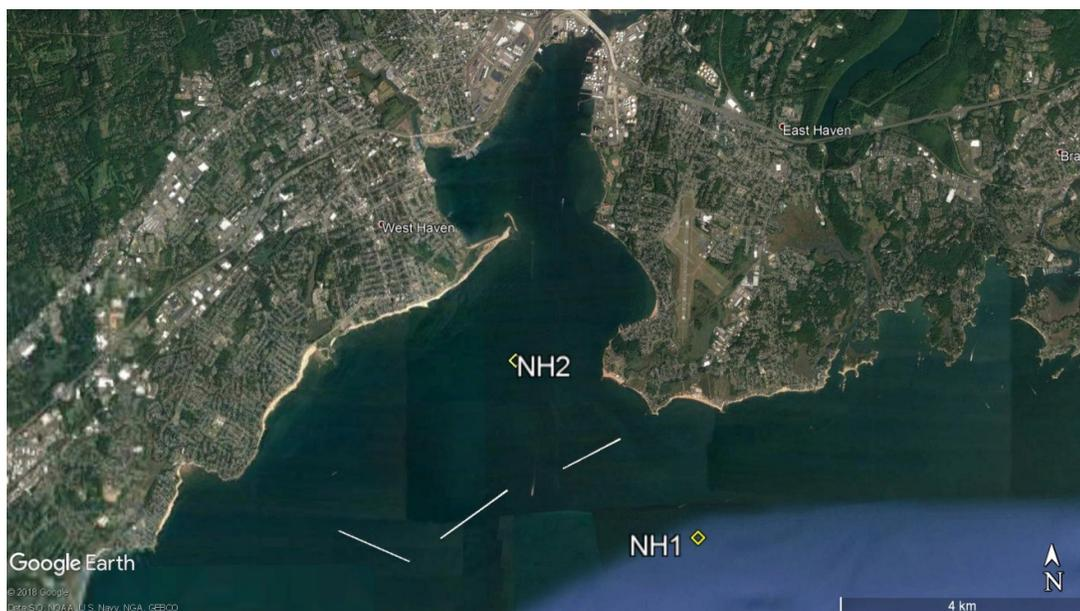
**Figure 1.** Locations of breakwater structures in front of New Haven Harbor are highlighted by white lines and ADCP locations inside and outside the harbor are identified by yellow boxes and labels. Image Source: “New Haven Harbor”. 41° 15′03.79″ N and 72° 55′20.36″ W. Google Earth. 23 September 2017. 18 June 2018.
