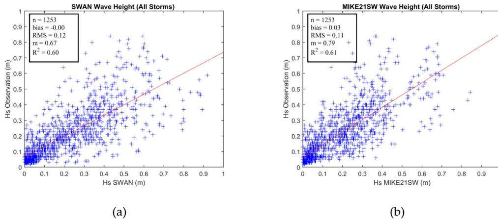
**Figure 10.** Comparison of scatter plot and statically parameter between observed and simulated significant wave heights from SWAN (a) and MIKE21SW (b) for all storms. There was no substantial difference between the performance of the models. *Bias* was better for SWAN and *RMS*, the slope best fitted line and *R*<sup>2</sup> were better for MIKE21SW.
