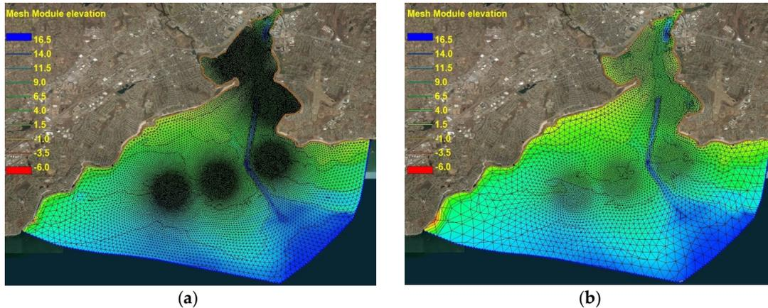
**Figure 3.** The optimum unstructured triangulate grids used for (a) SWAN with  $dx_{max} = 250$  m and  $dx_{min} = 25$  m and (b) MIKE21SW with  $dx_{max} = 500$  m and  $dx_{min} = 50$  m; SWAN required a finer grid to reach the optimum condition. The spatial smoothing of the grids is the same. The grids were refined around the breakwaters, three densification zones, and in the harbor.
