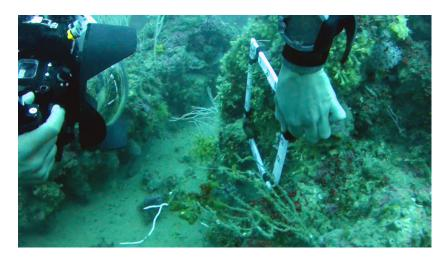
**Figure 3.** Diver holding the frame during the acquisition step (This approach is not recommended). The orientation phase is automatically performed using only the 36 coded targets printed on the quadrat. A post processing analysis of the residuals computed on measurements done manually will detect this problem (Photo: Olivier Bianchimani).
