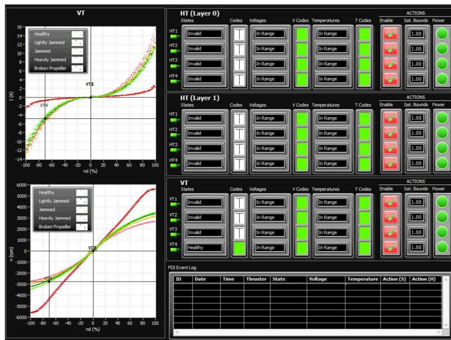
Figure 16. Thruster FDI result for thruster state = "Healthy".
