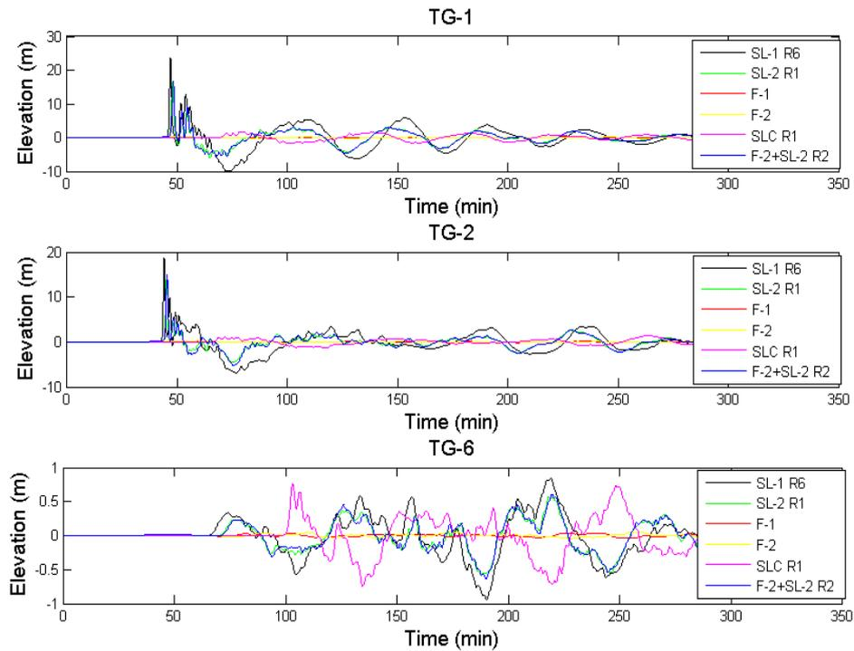
**Figure A2.** Computed time series of water elevations at tidal gauges TG-1, TG-2 and TG-6 for six of the tsunamigenic sources given in Tables 1 and 2. See Figure 3 for the location of the synthetic gauges. Initial water depths were 36, 33 and 36 m for TG-1, TG-2 and TG-6, respectively.
