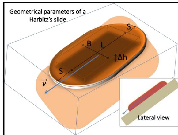
**Figure 2.** Sketch with the geometrical parameters defining the submarine landslide (following the formalism proposed by Harbitz, 1992, [36]). The adopted geometry is a box of length  $L$ , width  $B$  and maximum height  $\Delta h$ , and with an exponential smoothing over a distance  $S$  in the front and rear, and  $B/2$  on the flanks.
