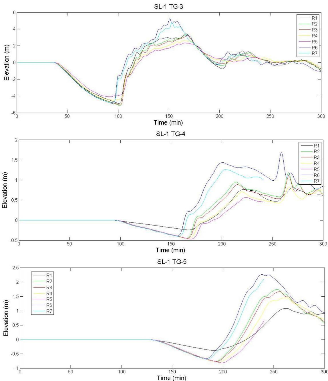
**Figure 5.** Computed time series of water elevations at tidal gauges TG-3, TG-4 and TG-5 for the submarine landslide SL-1, runs R1 to R7 (Table 1). See Figure 3 for the location of the synthetic gauges. Initial water depths were 9.0, 2.1 and 8.0 m for TG-3, TG-4 and TG-5, respectively.
