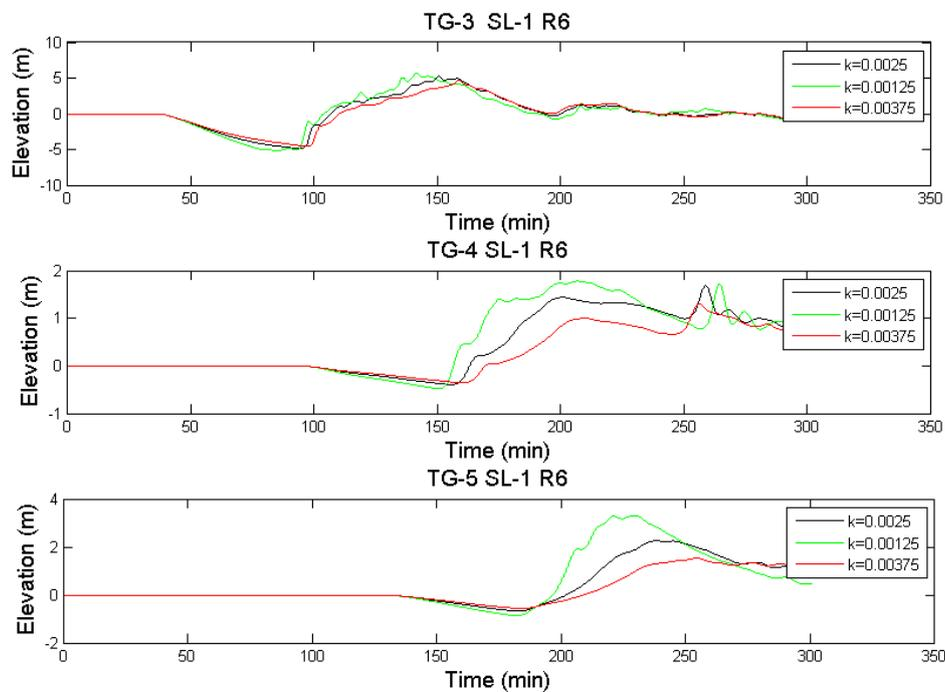
**Figure A3.** Computed time series of water elevations at tidal gauges TG-3, TG-4 and TG-5 for tsunami SL-1 R6 by increasing/decreasing by a 50% the nominal value of the friction coefficient (Equations (2)–(4)). See Figure 3 for the location of the synthetic gauges. Initial water depths were 9.0, 2.1 and 8.0 m for TG-3, TG-4 and TG-5, respectively.
