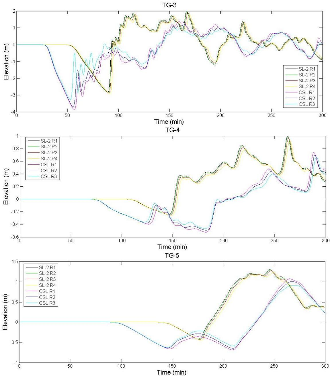
**Figure 6.** Computed time series of water elevations at tidal gauges TG-3, TG-4 and TG-5 for the submarine landslide SL-2, with runs R1 to R4; and CSL, with runs R1 to R3 (Table 1). See Figure 3 for the location of the synthetic gauges. Initial water depths were 9.0, 2.1 and 8.0 m for TG-3, TG-4 and TG-5, respectively.
