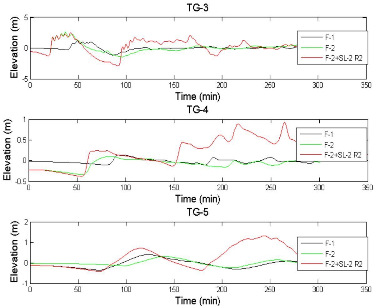
**Figure 8.** Computed time series of water elevations at tidal gauges TG-3, TG-4 and TG-5 for the geological faults F-1, F-2, and the double source F-2 + SL-2 R2 (Table 1). See Figure 3 for the location of the synthetic gauges. Initial water depths were 9.0, 2.1 and 8.0 m for TG-3, TG-4 and TG-5, respectively.
