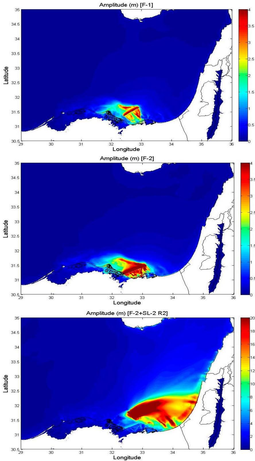
**Figure 7.** Computed maximum amplitude for water elevations (m) due to geological faults F-1, F-2 and the double source F-2 + SL-2 R2. Source parameters are presented in Table 1. Simulation time is 5 h.
