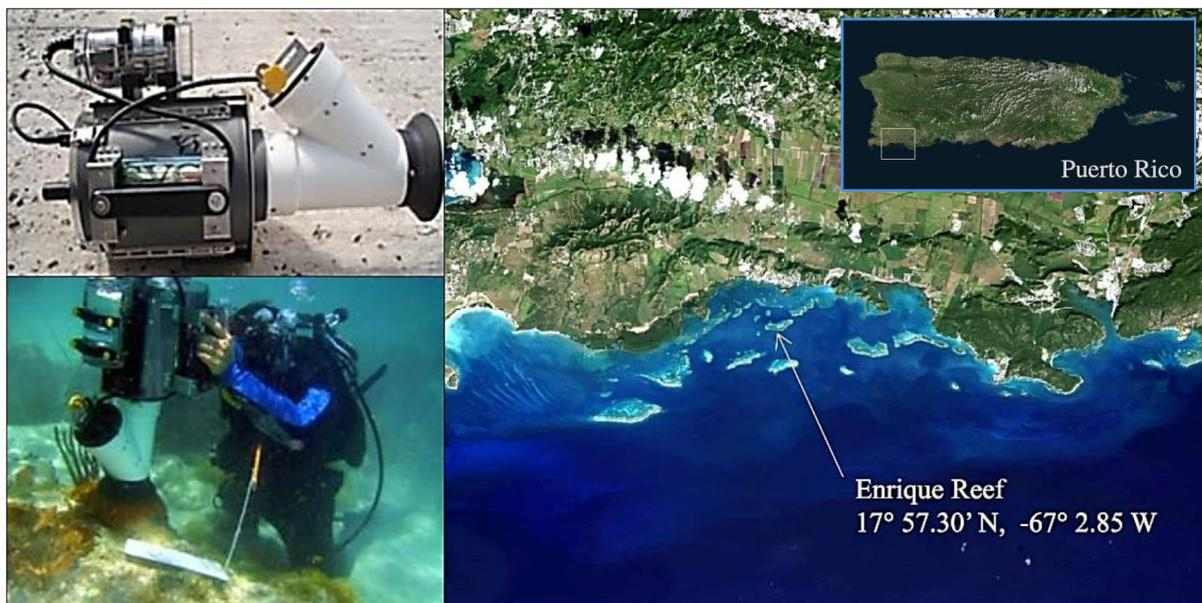
**Figure 1.** The GER-1500 spectrometer in underwater housing with attached illumination (left) and a map of the study location off the coast of southwestern Puerto Rico (right).
