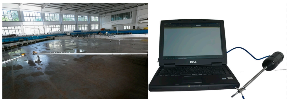
Figure 9. Basin current-generation pump and NDV high-precision acoustic Doppler velocimeter.
