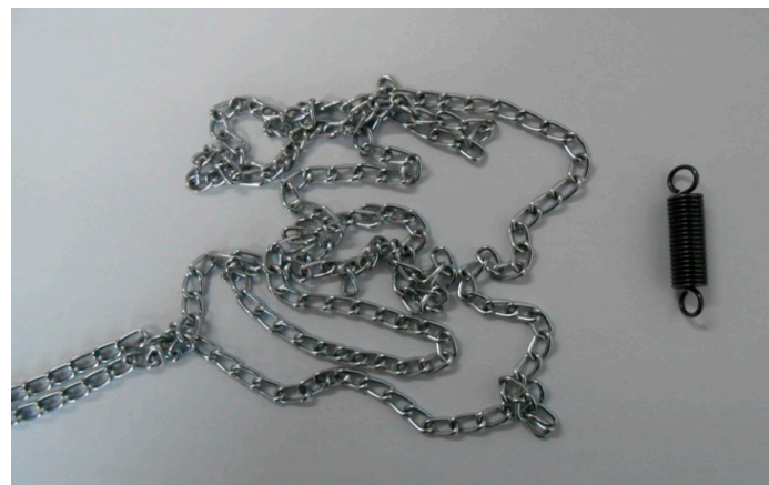
Figure 6. Anchor chain modeling using fine chains and calibrated springs.
