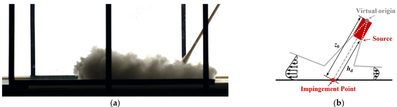
Figure 5. Morphology non-axisymmetric bottom plume: (a) Image from case A3 ( \alpha = 60^\circ ), and (b) Parameters at the moment of impact.
