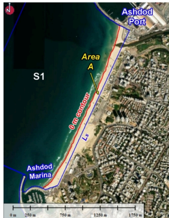
Figure 14. Geometric definition of the variables used in the Mean Width (MW) shoreline analysis for Segment S1. The example is shown on a satellite image overlaid with the elevation-derived 0 m ILSD contour for 2025 (red). Segment S1 extends from the root of the Ashdod Marina LBW northward to the root of the Ashdod Port MBW. The analysis polygon is enclosed by the shoreline (0 m ILSD contour), a fixed straight landward baseline ( L_s ), and fixed northern and southern segment boundaries (blue). The polygon area ( A ) is used to calculate the Mean Width (MW) by dividing A by the fixed baseline length ( L_s ). Background image: Maxar (Vivid) satellite imagery, acquired on 18 September 2023. © Maxar Technologies. Used with permission.
