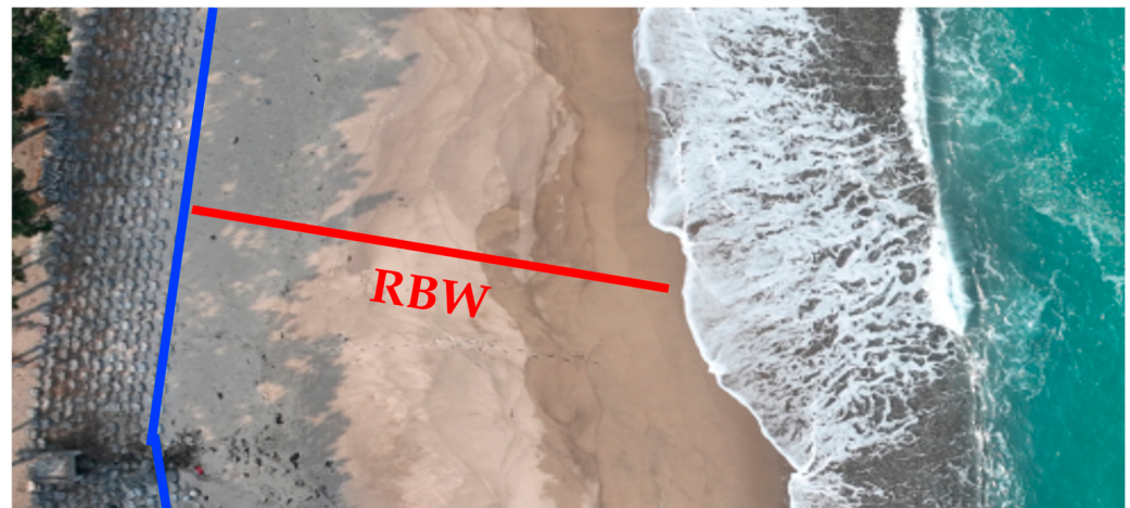
Figure 2. Conceptual definition of Remaining Beach Width (RBW) on an orthomosaic base image. The blue line denotes the coastal baseline, and the red segment denotes RBW measured from the coastal baseline to the landward runup front detected from time resolved CCTV imagery.
