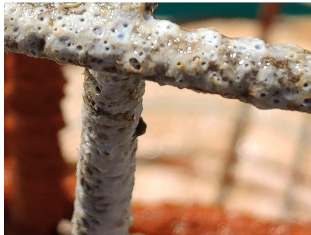
Figure 6. Appearance of one of the calcareous layers obtained in this work by electrolysis in sea water, immediately after hoisting from sea water. (Photo: C. Antón).
