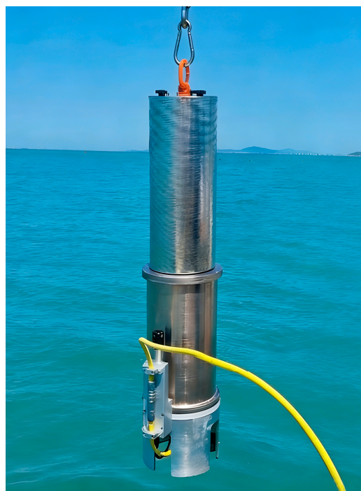
Figure 2. Automatic seawater in situ fidelity sampler.
