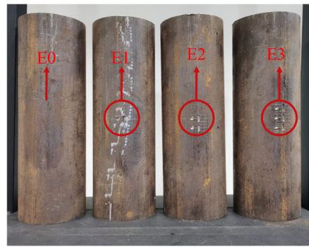
Figure 18. Four distinct damage scenarios.
