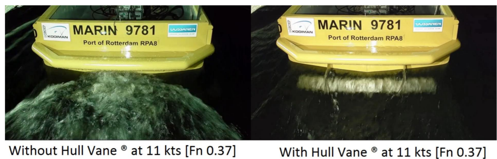
Figure 3. Comparison between wave formation with and without Hull Vane®.
