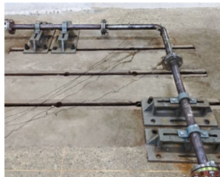
Figure 20. The experimental model of the elbow pipe with flanges (water-filled).
