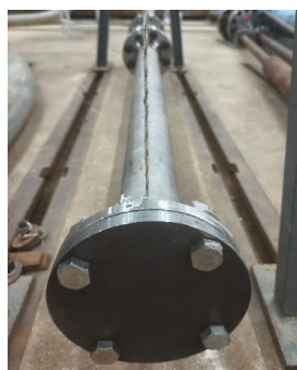
Figure 18. The experimental model of the pipe (water-filled).
