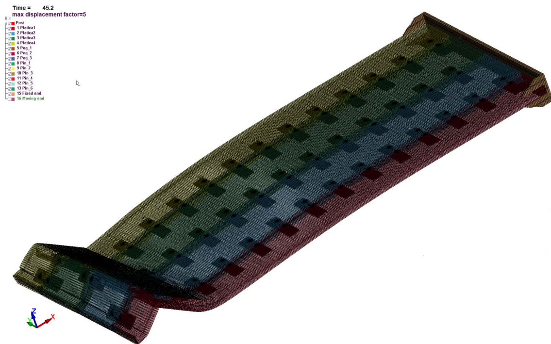
Figure 6. Deformed models at the time instance of maximal load for bending (top) and compression (bottom)—Joint 1 (Kyrenia).
