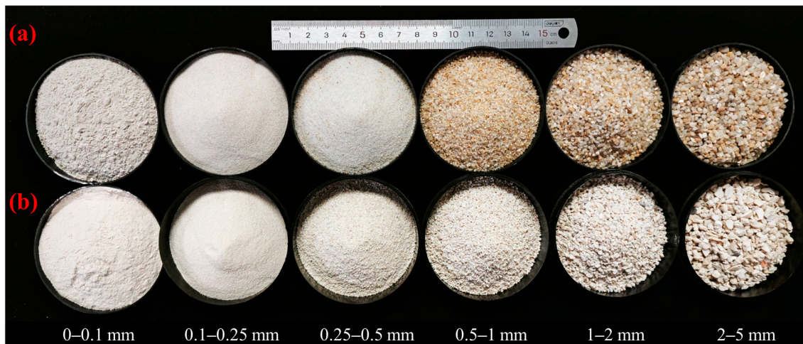
Figure 2. Six groups of quartz sand (QS) and coral sand (CS) samples: (a) QS; (b) CS.
