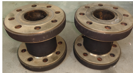
Figure 8. FRF pipe specimens for axial stiffness testing.
