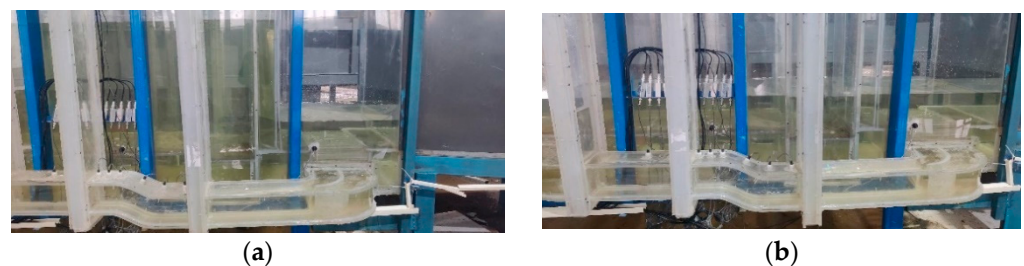
Figure 13. Chamber emptying process of the ship lock water conveyance system. (a) Before chamber emptying; (b) after chamber emptying.
