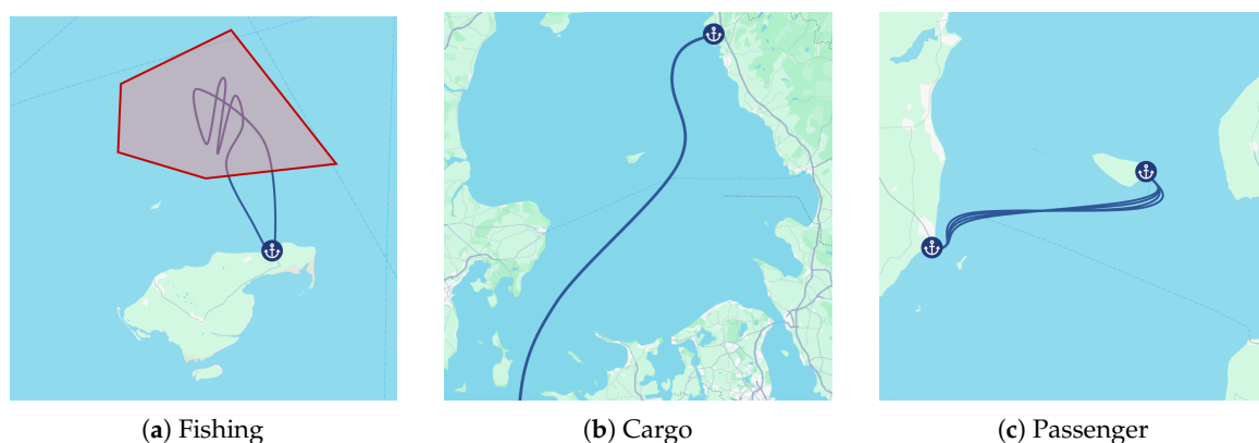
Figure 1. Schematic diagram of the spatiotemporal characteristics of different ship trajectory types. The blue lines represent the trajectories, and the red areas indicate the fishing ban zones. To ensure clarity, we have simplified and abstracted the trajectory representation while preserving key motion patterns.
