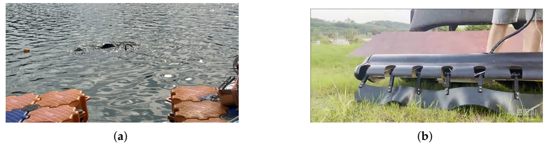
Figure 15. The process of the autonomous survey mission experiment: (a) Robot moving in lake. (b) Robot slithering on land.
