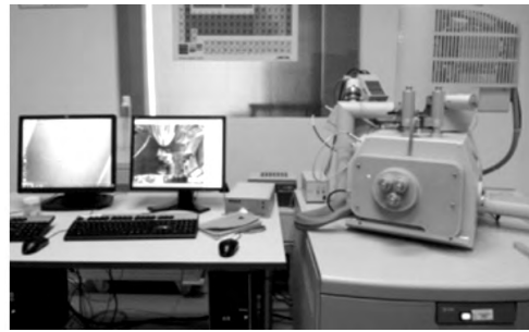
Figure 2. Scanning electron microscope of the FEG650 type.
