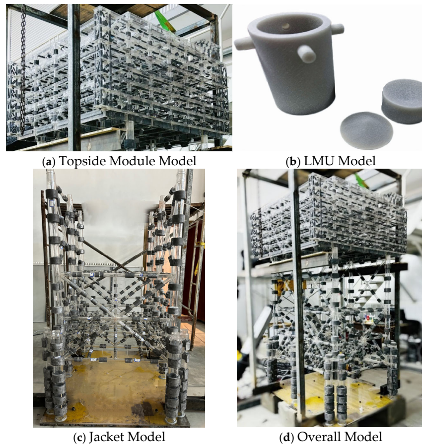
Figure 1. Offshore converter station platform model.
