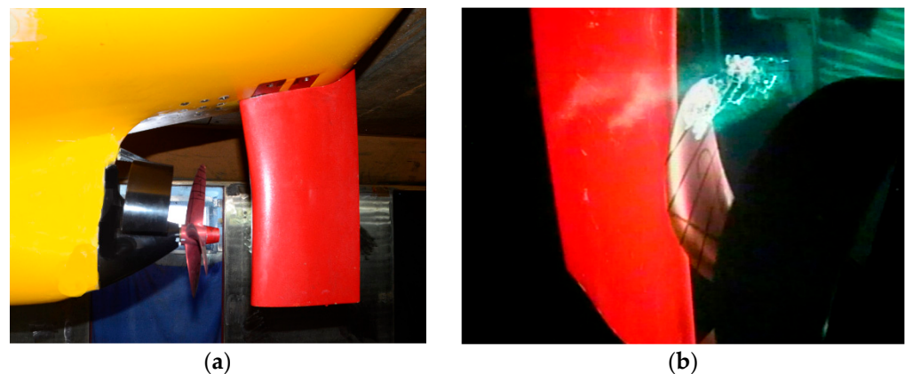
Figure 25. Experimental photos of the original propeller: (a) the installation photo; (b) the cavitation photo.
