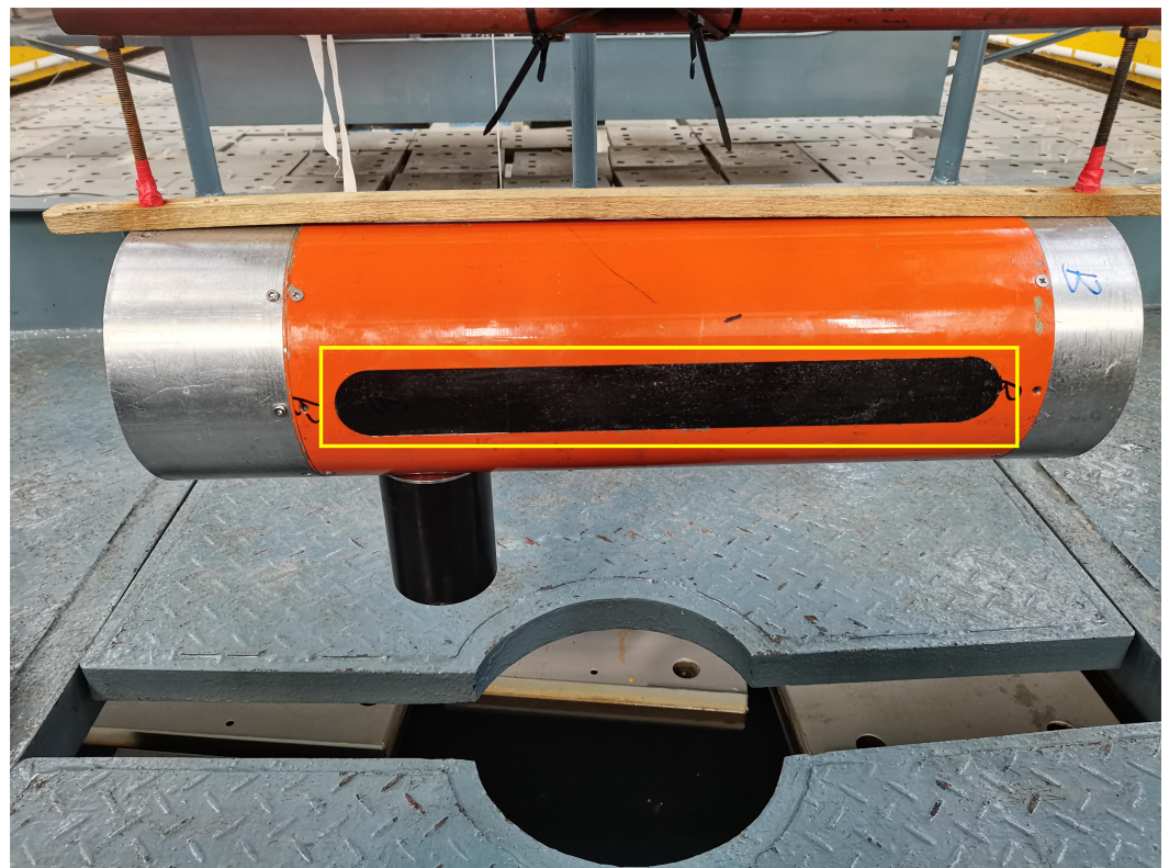
Figure 7. Underwater acoustic transducer array (in the yellow box).
