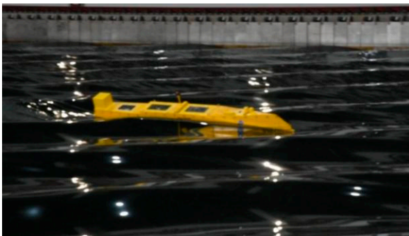
(a) pure loss of stability ( Fn = 0.3 )
