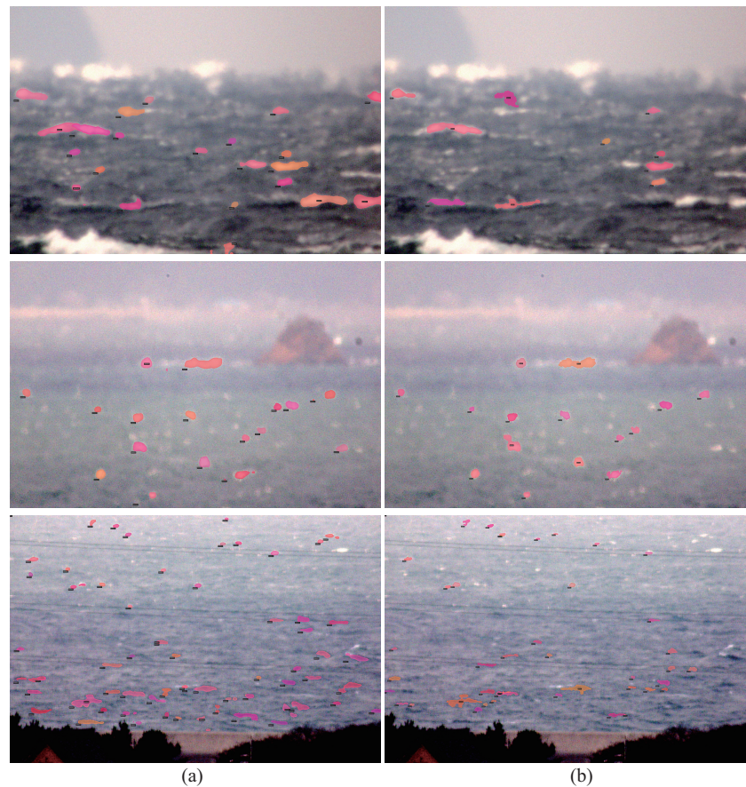
Figure 9. Comparison of sea wave detection results, column (a) shows the results described in this paper, column (b) shows results of [52]. From top to bottom are the images shoot from 14–20 km, 8–14 km and 4–10 km.
