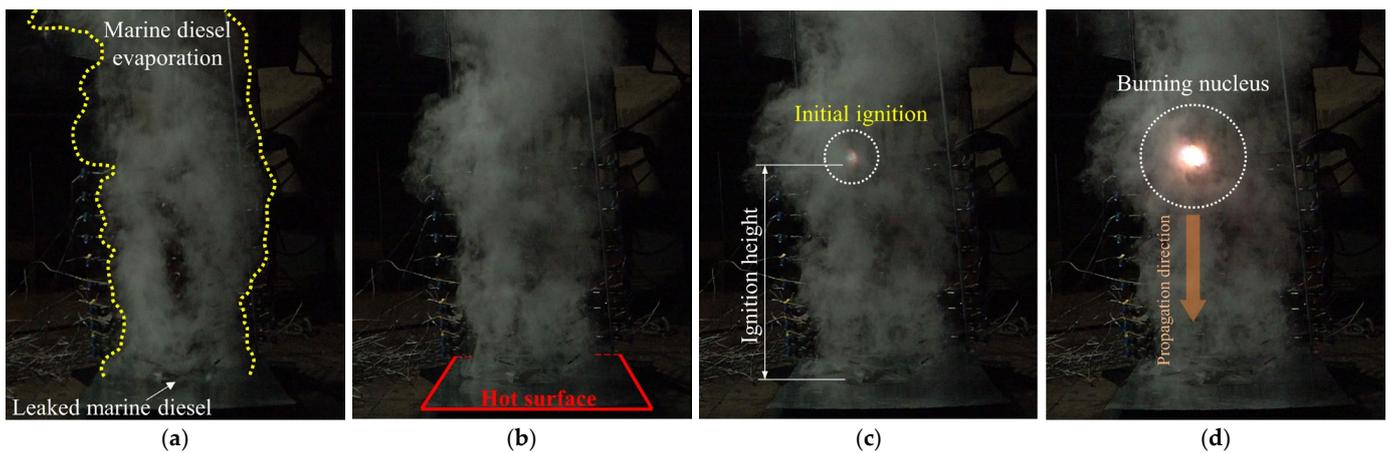
**Figure 2.** The initial ignition of marine diesel leaking onto the hot surface of a ship engine system. (a)  $t = 3.108$  s; (b)  $t = 3.675$  s; (c)  $t = 3.725$  s; (d)  $t = 3.733$  s.
