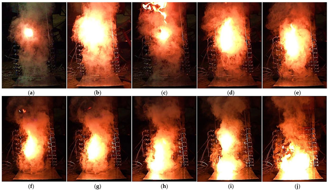
**Figure 4.** Flame propagation from ignition position to the hot surface. (a)  $t = 3.741$  s; (b)  $t = 3.758$  s; (c)  $t = 3.933$  s; (d)  $t = 4.091$  s; (e)  $t = 4.174$  s; (f)  $t = 4.299$  s; (g)  $t = 4.333$  s; (h)  $t = 4.424$  s; (i)  $t = 4.541$  s; (j)  $t = 4.673$  s.
