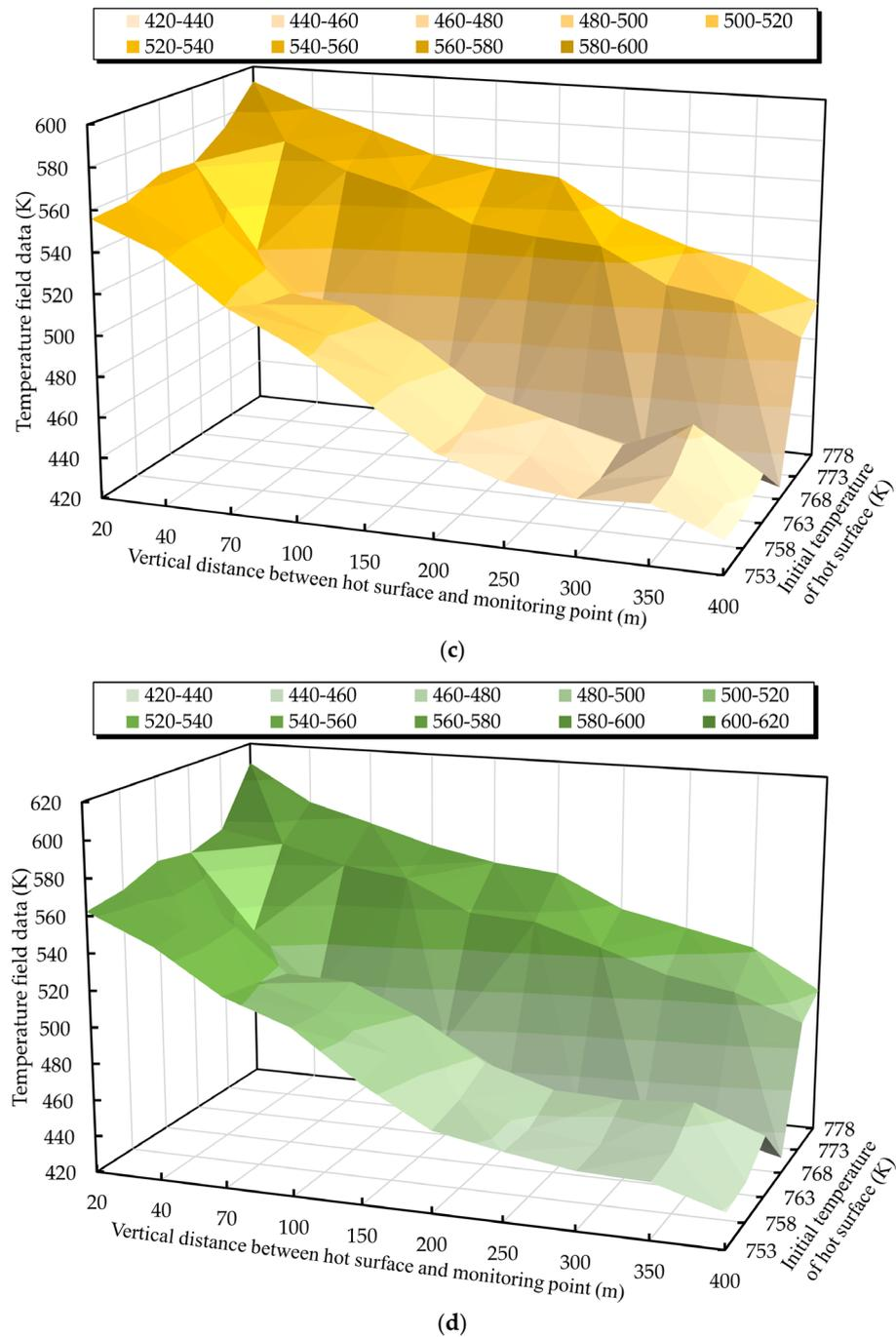
**Figure 5.** Temperature field distribution induced by marine diesel HSI. (a)  $t = 3.011$  s; (b)  $t = 5.132$  s; (c)  $t = 7.312$  s; (d)  $t = 9.036$  s.
