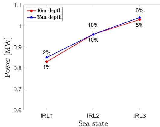
**Figure 8.** Power output of the  $4 \times 4$  array layout ( $d = 150$  m) for the water depths 46 m and 55 m and the irregular sea states IRL 1 to 3. The percentages are the interaction factors indicating the additional power generation due to interaction effects.
