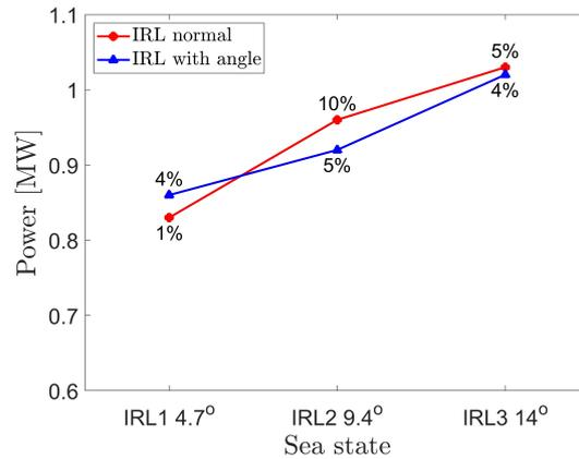
**Figure 12.** Power output of the  $4 \times 4$  array layout ( $d = 150$  m) for different wave directions and the irregular sea states IRL 1 to 3. The percentages are the interaction factors indicating the additional power generation due to interaction effects.
