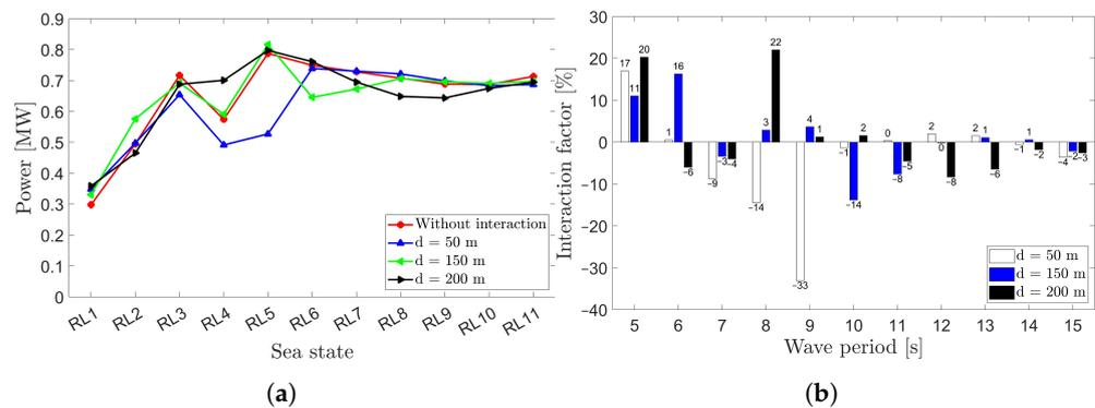
**Figure 13.** (a) Power output of the  $4 \times 4$  array layout for different WEC distances for regular wave conditions RL 1 to 11. (b) Interaction factors for different WEC distances under regular wave conditions RL 1 to 11.
