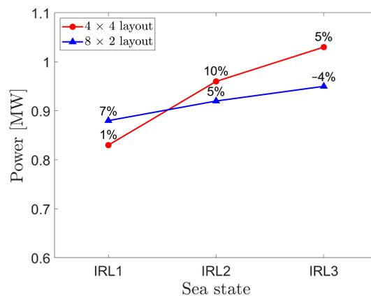
**Figure 9.** Power output of the  $4 \times 4$  and  $8 \times 2$  array layouts ( $d = 150$  m) for the irregular sea states IRL 1 to 3. The percentages are the interaction factors indicating the additional power generation or power reduction due to interaction effects.
