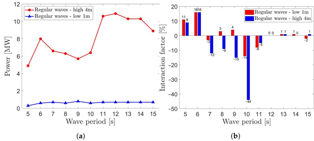
**Figure 6.** (a) Power output of the  $4 \times 4$  array layout ( $d = 150$  m) for the regular wave conditions RL 1 to 11 and RH 1 to 11; see Table 3 for details. (b) Interaction factors for the cases presented in (a); see the text for details.
