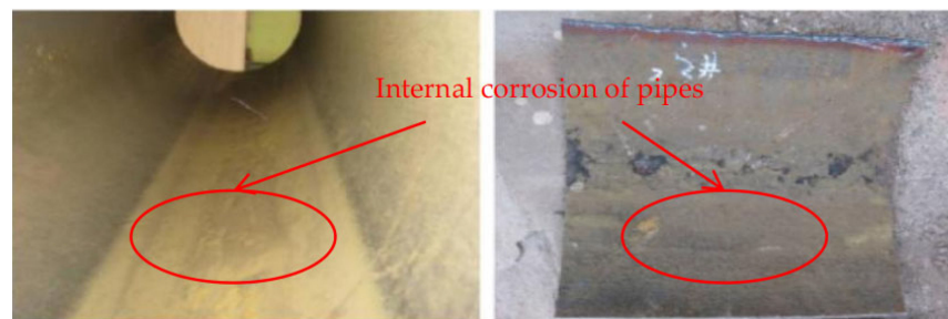
Figure 1. Pipeline corrosion morphology.
