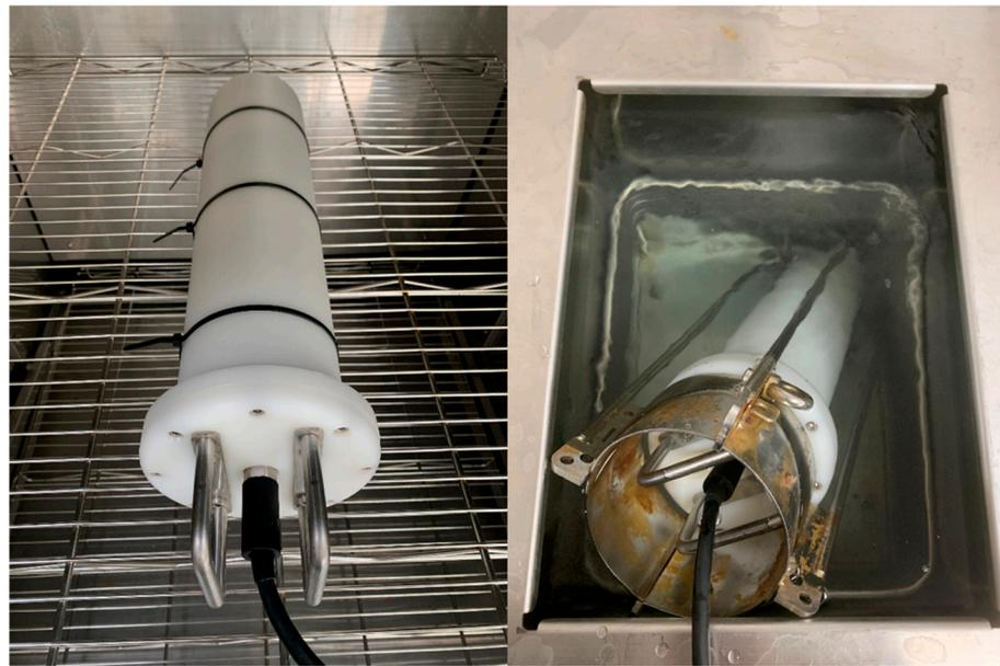
**Figure 2.** The seawater radioactivity sensor placed as a whole in the air temperature experiment box (left) and the water temperature experiment box (right).
