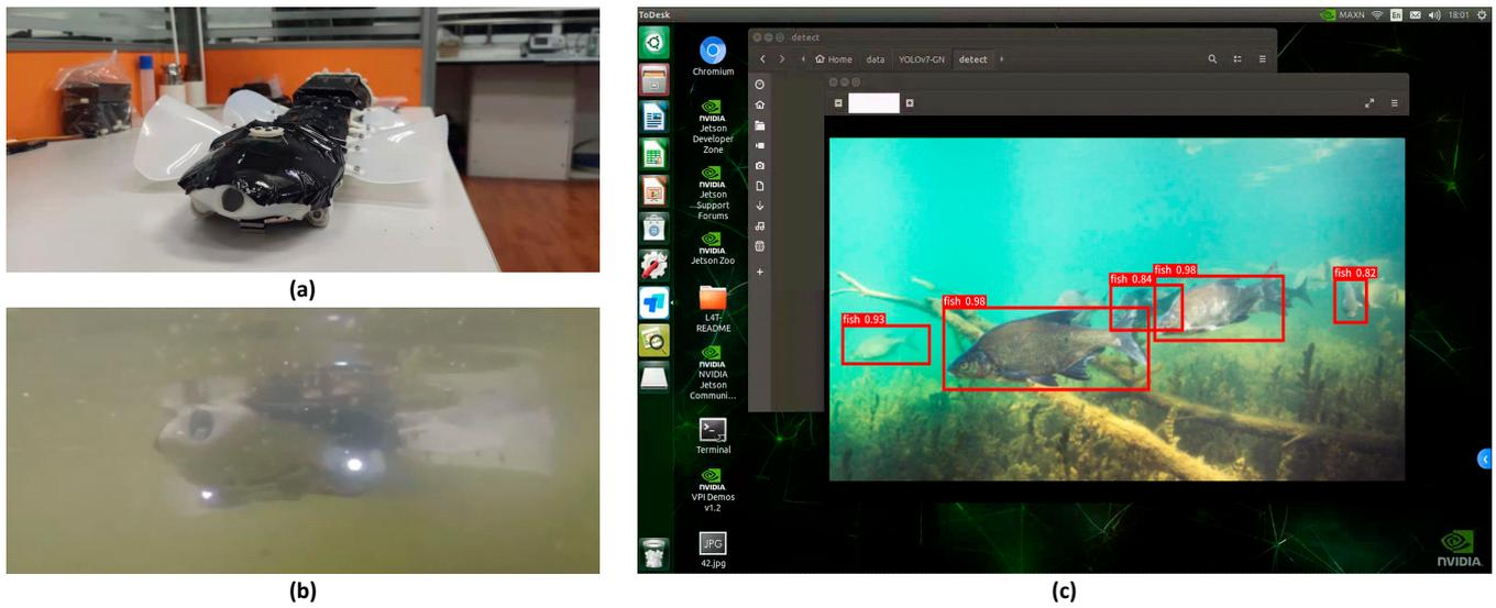
**Figure 21.** Real-world testing of the biomimetic flatworm robot. (a) Photograph of the robot. (b) The underwater working state of the robot. (c) Ubuntu recognition result interface.
