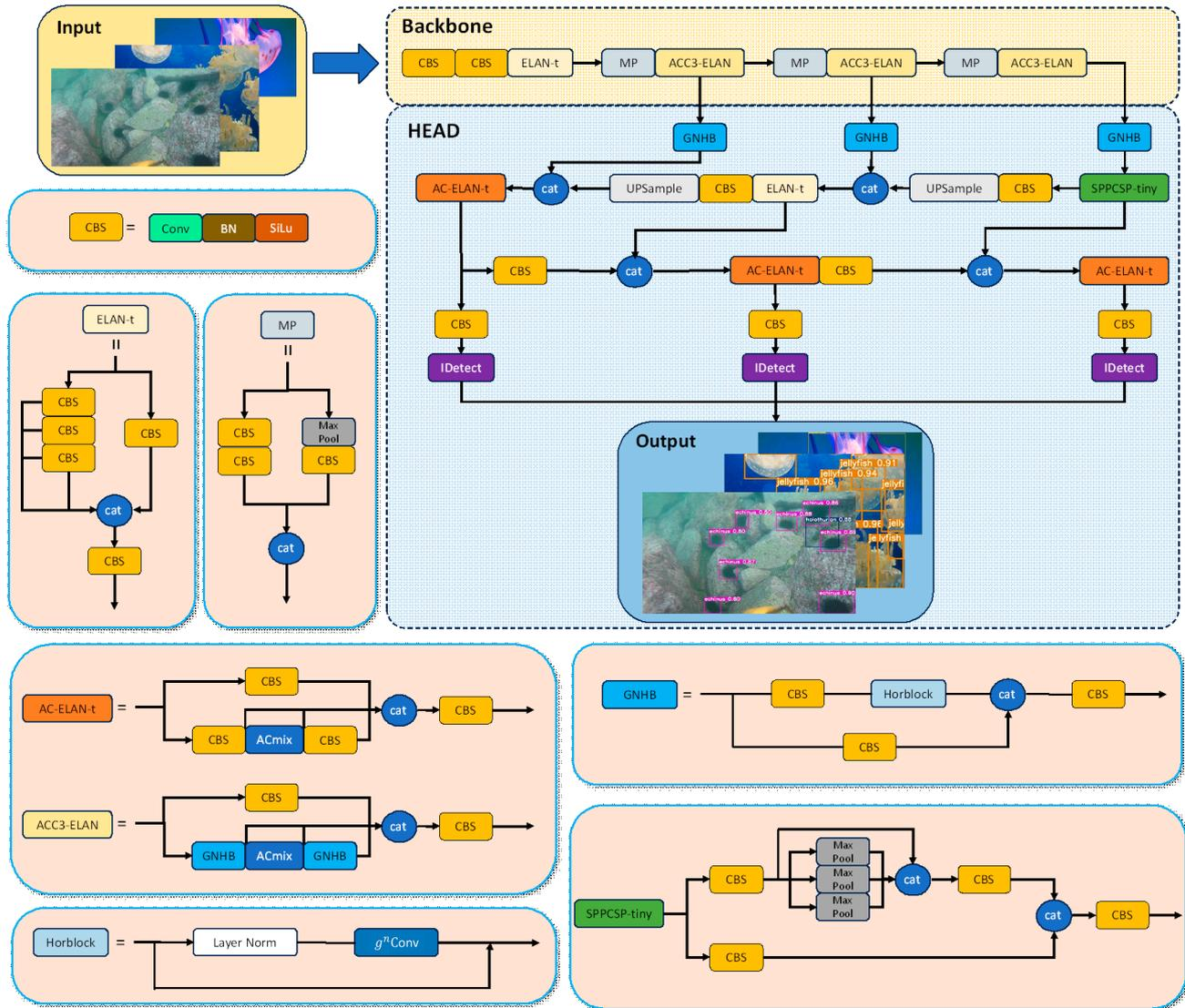
Figure 6. The overall network structure of YOLOv7-GN.
