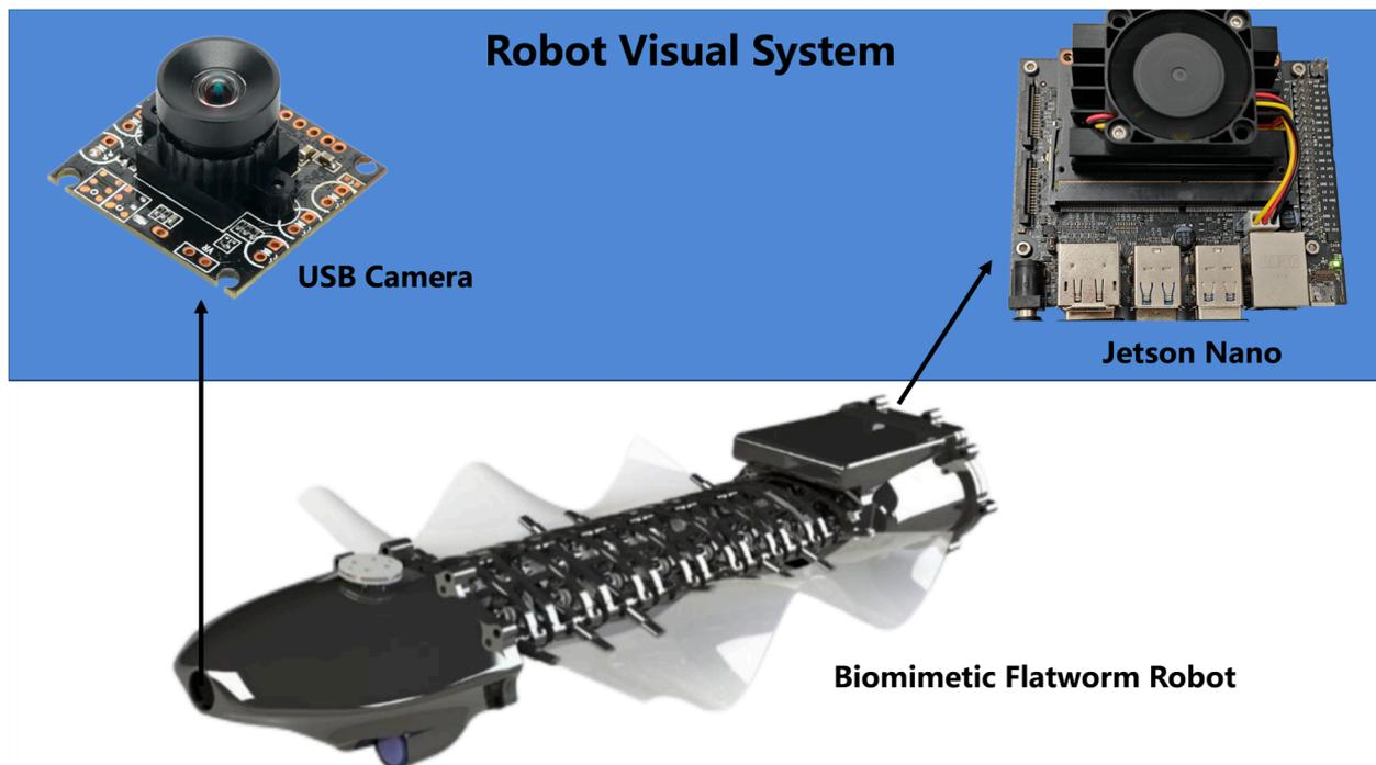
**Figure 20.** Biomimetic flatworm underwater robot vision system, consisting of a USB camera in the head and a Jetson Nano master control in the tail.
