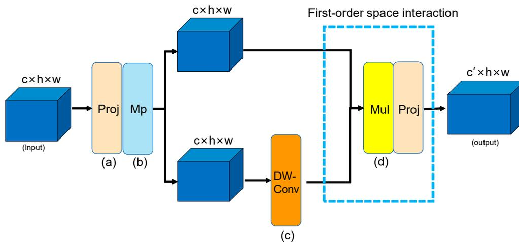
**Figure 7.** Principles of first-order spatial interaction. (a) Linear projection layer, which can map the input  $c$ -channels to any dimension. (b) Matrix partitioning splits the input into two outputs of equal size. (c) Depth-wise convolution. (d) Matrix Multiplication, which is used to calculate the product between two matrix.
