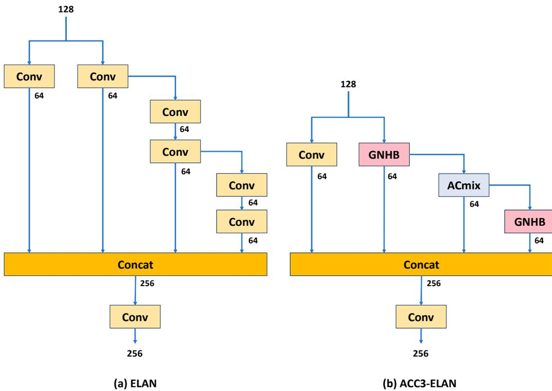
Figure 9. Structures of ELAN and ACC3-ELAN. (a) ELAN. (b) ACC3-ELAN.
