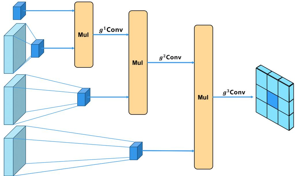
**Figure 8.** Conv. where Mul is Multiplication, which realizes arbitrary order spatial information interaction by using recursive gated convolution.
