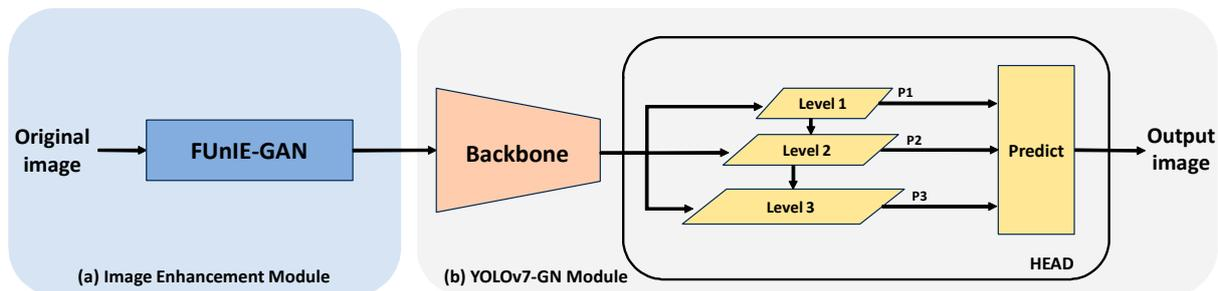
**Figure 4.** Complete architecture of the proposed solution. (a) Image enhancement module. (b) YOLOv7-GN module.
