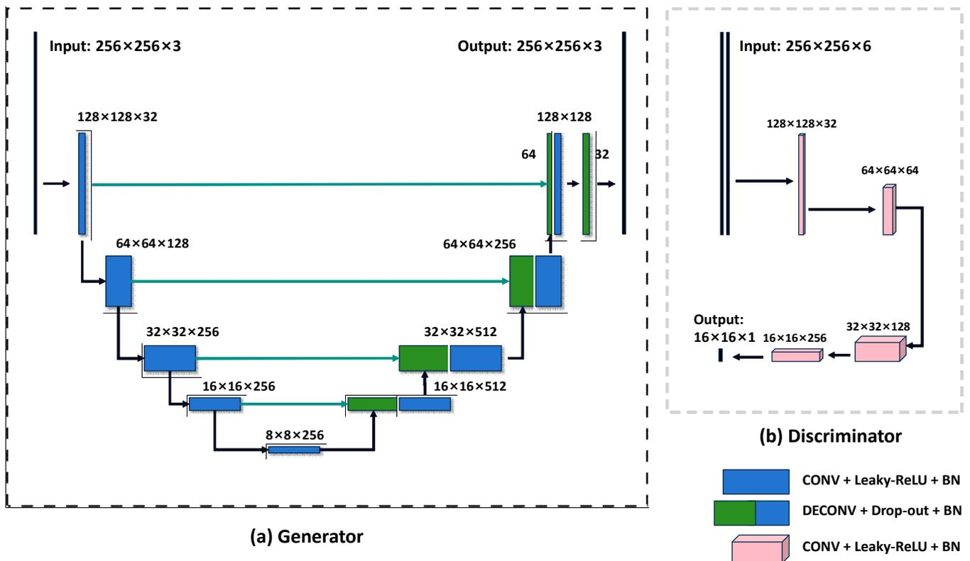
**Figure 5.** The overall network structure of FUnIE-GAN is divided into two parts: Generator and Discriminator. (a) Generator: a fully convolutional network using the U-net structure, in which the encoder and decoder have 5 convolutional layers each, and the decoder uses inverse convolution. (b) Discriminator: a Markovian PatchGAN is used to seek similarity between local texture and content.
