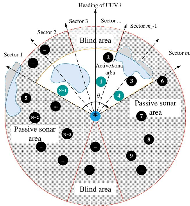
Figure 5. Dynamic interaction framework based on active sonar.
