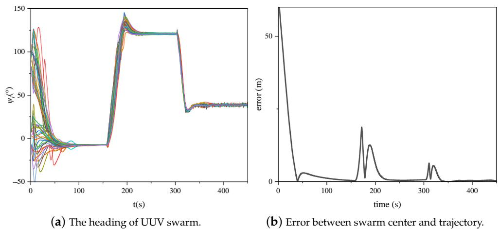
Figure 9. The heading of UUV swarm and error between swarm center and given trajectory.
