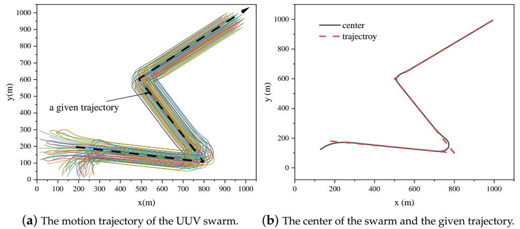
Figure 8. Route tracking results of the UUV swarm.
