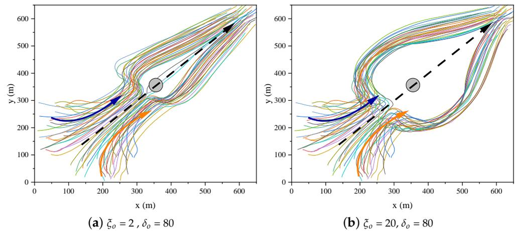
Figure 12. The effect of  $\zeta_o$  on obstacle avoidance.
