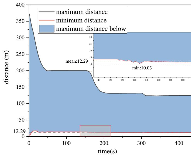
**Figure 10.** The max–min distances between UUVs.
