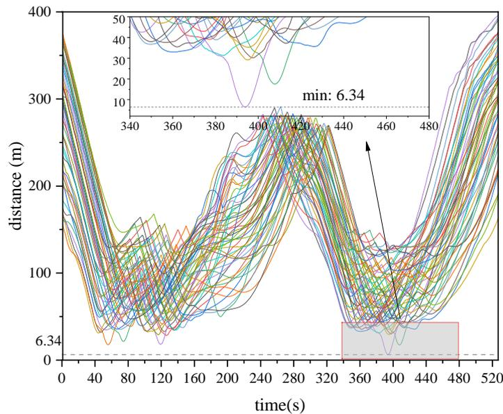
Figure 15. The minimum distance from UUVs to obstacles.
