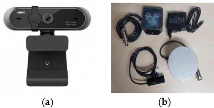
Figure 2. A sensor system in the lab-scale GTSU system: (a) APC930 QHD webcam; (b) Velodyne LiDAR VLP-16 sensor.
